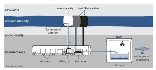
This is a non-entry method, which means mining is carried out from headings in the basement rock below the deposit, so employees are not exposed to the ore. This mining approach is highly effective at managing worker exposure to radiation levels. Combined with ground freezing and the cuttings collection and hydraulic conveyance system, jet boring reduces radiation exposure to acceptable levels that are below regulatory limits.
